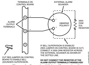
Figure 5. Sounder Wiring (Supervised)
